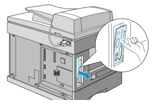
7 Remove the plates covering the network port and LED slots from the port cover.
